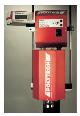
Drive and Control Unit PT 7000 with programming unit RECO  $^{\circledR}$  RP 502
